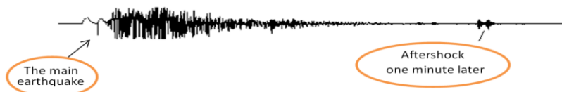
Figure7. Simple image of the earthquake and aftershock recorded by seismograph for the earthquake of Southern California (1992) with a magnitude of 7.3 Richter
