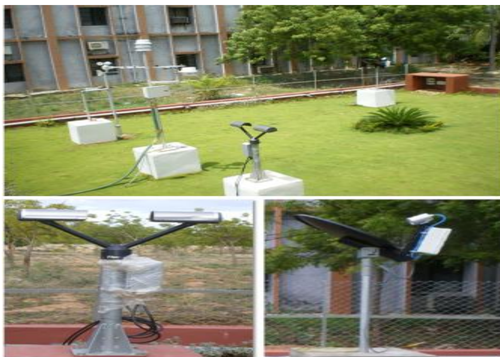
Figure 2.2. Photograph of the observational showing ground based instruments Parsivel disdrometer, Automatic Weather Station (AWS) and Micro Rain Radar (MRR).
