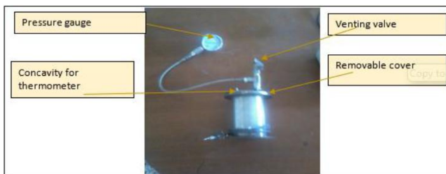
Figure1. The homemade design of hydrothermal autoclave
