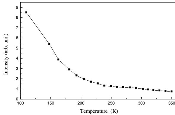
**Fig4.** Variation of LED intensity with temperature at a driving current of 15 mA
