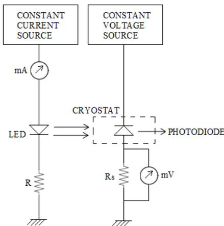
Fig1. Schematic diagram of the experimental set up used for the photo-voltage ( $V_{ph}$ ) measurement
