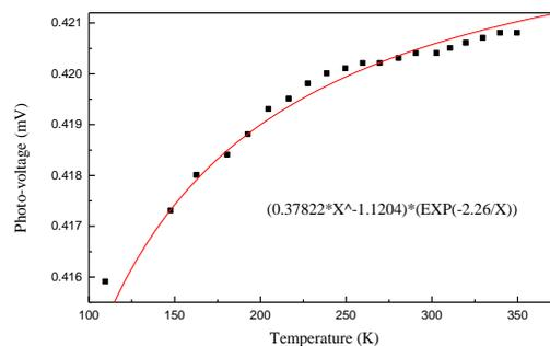
Fig2. Variation of the photodiode's output with temperature for fixed illumination incidents on it. Numerical fit, continuous line according to Eq. (3). The solid square indicates the experimental points
