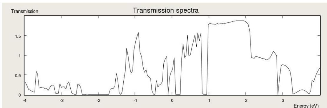
**Fig7.** Transmission Spectrum of Graphene adsorbed with Beryllium at -2v
