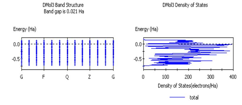
**Fig6.** Band structure and Density of States of Graphene adsorbed with one Beryllium atom
