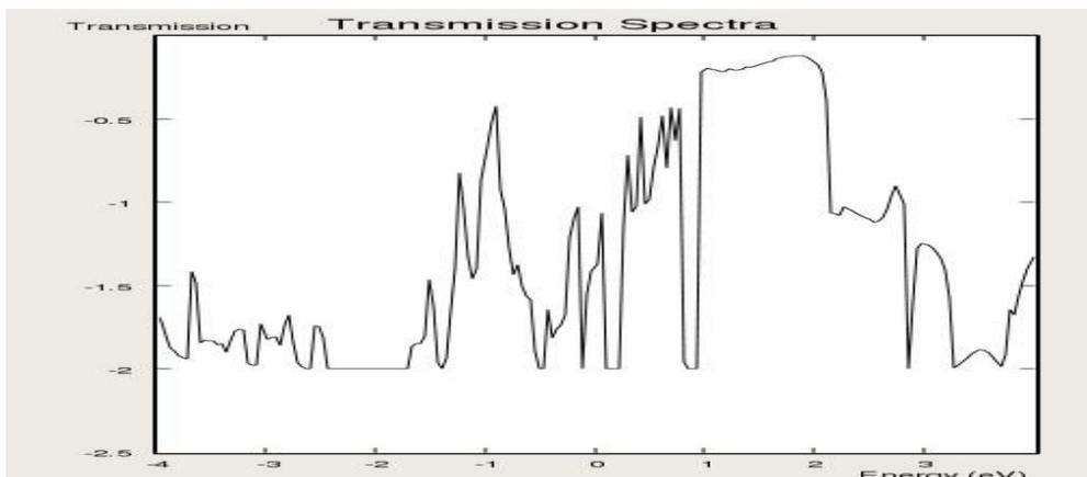
Fig4. Pure Graphene transmission spectra with -2 bias Voltage
