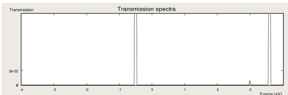
**Fig8.** Transmission Spectra of Graphene adsorbed with Beryllium at 2V
