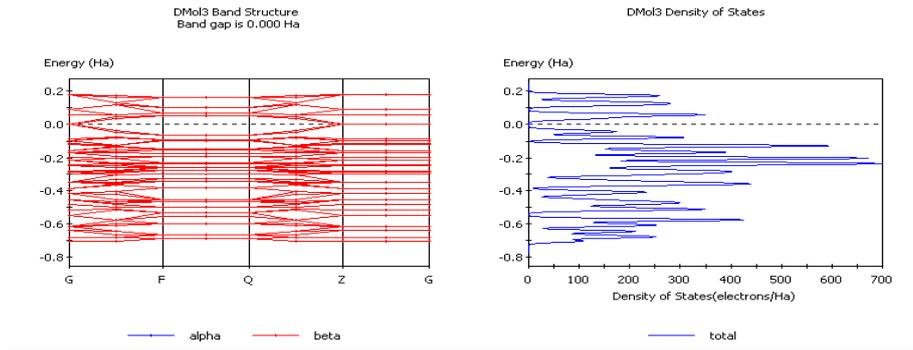
Fig3. Band structure and Density of States of pure Graphene
